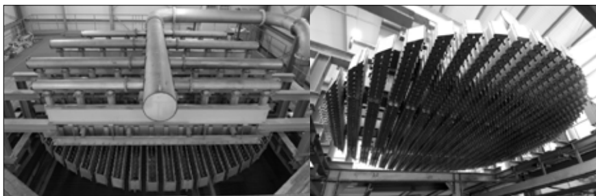
Figure 4 Large scale DT-S distributor in Raschig's test facility in Germany
